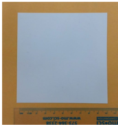
Sealing glass tapes are available in various sizes (Pictured: 10 cm × 10 cm tape)
